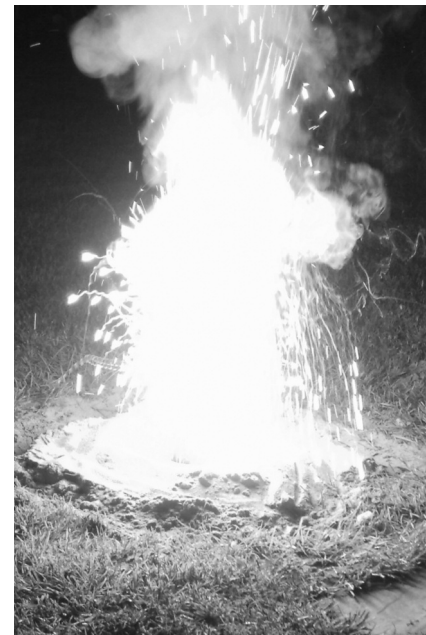
The thermite reaction is very hot, but it is also very slow compared to high explosives.
